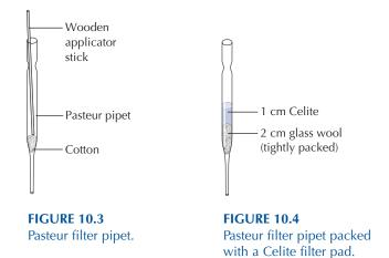
microclamp to hold the filter pipet in a vertical position for the filtration and place a small Erlenmeyer flask underneath it. Use another Pasteur pipet to transfer the mixture being filtered to the filter pipet. The drying agent or solid impurities will adhere to the cotton. Use a clean Pasteur pipet to add 1–2 mL of fresh solvent to the filter pipet to rinse all desired material from it and collect the rinse in the same Erlenmeyer flask.
