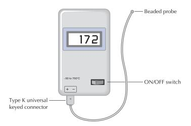
**FIGURE 5.11** Digital thermometer.
