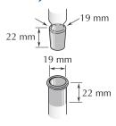
FIGURE 4.3 Dimensions of ₹ 19/22 ground glass joints.
