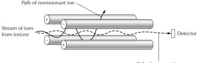
**FIGURE 23.4** Quadrupole mass filter.
