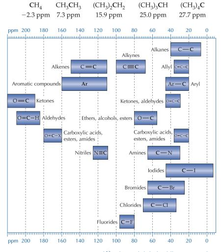
**FIGURE 22.4** Approximate regions of <sup>13</sup>C chemical shifts for different types of carbon atoms in organic compounds.
