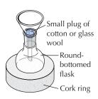
FIGURE 12.3 Filtration of drying agent from an organic liquid when no solvent is present.
