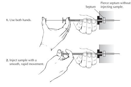
FIGURE 19.10 Injecting the sample into the column.
