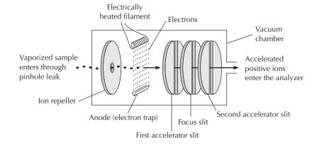
**FIGURE 23.2** Electron impact (EI) ionization chamber.
