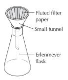
**FIGURE 12.2** Filtration of drying agent from a solution when the solvent will be evaporated.
