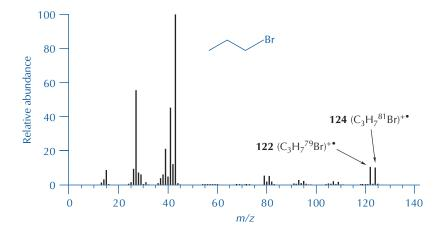
FIGURE 23.7 Mass spectrum of 1-bromopropane.
