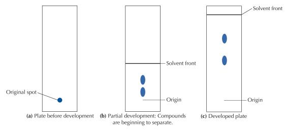
FIGURE 17.2 Steps in development of a TLC plate.
