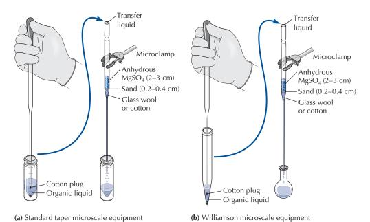
**FIGURE 12.4** Using microscale equipment and a Pasteur filter pipet containing anhydrous MgSO<sub>4</sub> to dry an organic liquid or solution.
