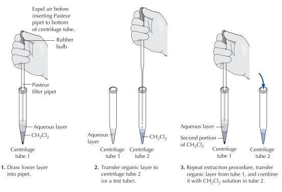
FIGURE 11.10 Extracting an aqueous solution with an organic solvent denser than water.
