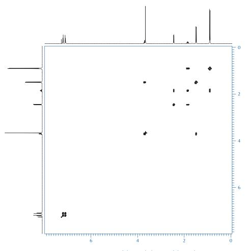
FIGURE 22.21 2D (H,H) COSY spectrum of the methyl ester of ibuprofen.
