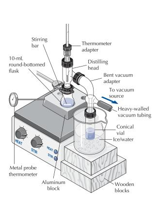
**FIGURE 13.28** Short-path standard taper microscale apparatus for vacuum distillation.
