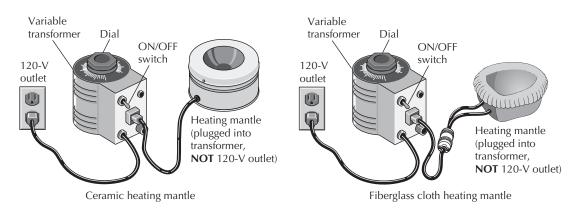
FIGURE 6.1 Heating mantle and variable transformer. (Note: The transformer dial is calibrated in percentage of line voltage, **not** in degrees.)
