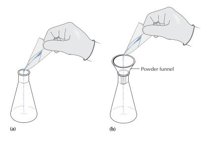
**FIGURE 15.2** Two ways to add a solid to an
