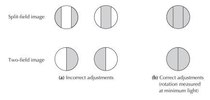
**FIGURE 16.5** Representative images in the light field of a manual polarimeter.
