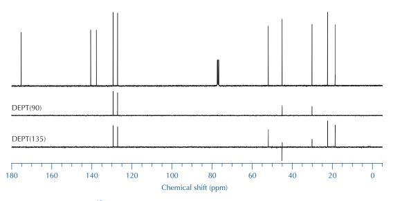
FIGURE 22.19 90-MHz <sup>13</sup>C NMR, DEPT(90), and DEPT(135) spectra of the methyl ester of ibuprofen.
