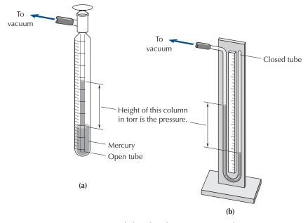
**FIGURE 13.23** Two types of closed-end manometers used in vacuum distillations.
