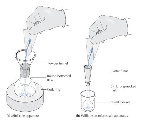
FIGURE 5.3 Transferring solids with a powder funnel.
