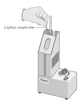
holds the sample. The capillary tube fits into one of three sample chambers in the heating block; multiple chambers allow simultaneous determinations of three melting points. A cylindrical cavity in the top of the heating block holds the thermometer, a light illuminates the sample chamber, and an eyepiece containing a small magnifying lens facilitates observation of the sample. A digital thermometer can also be used with a Mel-Temp apparatus.
