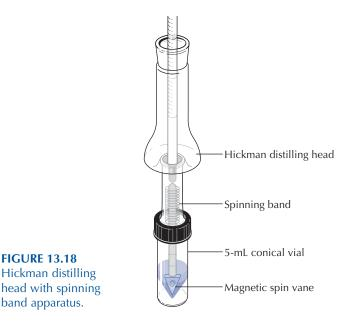
Microscale Fractional Distillation into a thin film and forces the rising vapors into contact with the descending condensate. The result is a large increase in the number of vaporization/condensation equilibria in the column. Spinning-band columns can have more than 100 theoretical plates and can be used to separate liquids that have a boiling-point difference of only a few degrees.
