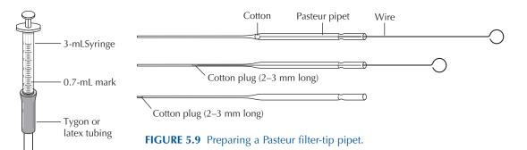
*Pasteur filter-tip pipets.* Volatile organic liquids tend to drip from a Pasteur pipet during transfers because the vapor pressure increases as your fingers warm the rubber bulb. If a small plug of cotton is pushed into the tip of the pipet, a liquid can be transferred from one container to another without dripping.
