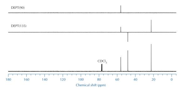
**FIGURE 25.6** 90-MHz <sup>13</sup>C NMR, DEPT(90), and DEPT(135) spectra of unknown compound for problem 5.
