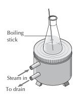
**FIGURE 15.3** Heating a solution on a steam bath.
