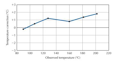
**FIGURE 5.12** Thermometer calibration graph.
