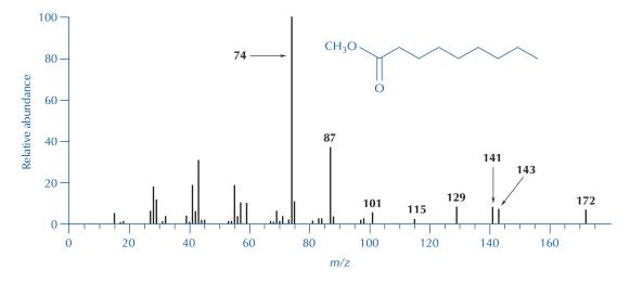
FIGURE 23.14 Mass spectrum of methyl nonanoate.
