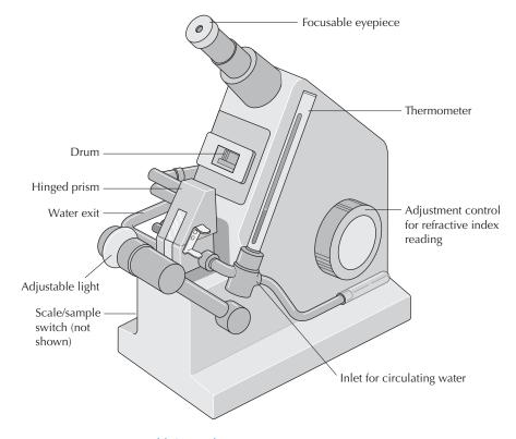
FIGURE 16.2 Abbé-3L refractometer.
