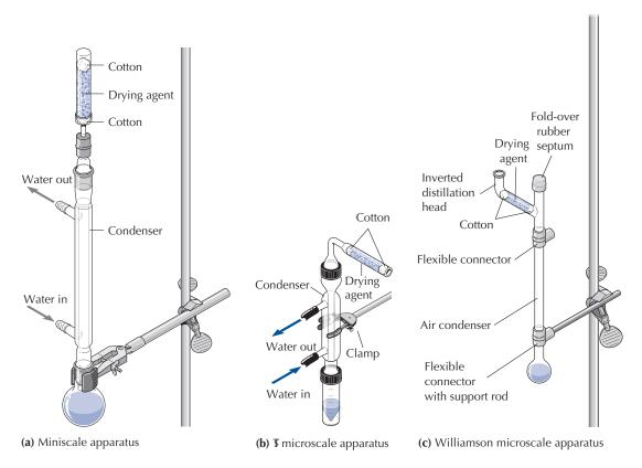
**FIGURE 7.2** Refluxing under anhydrous conditions.
