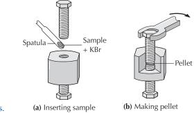
**FIGURE 20.10** Preparation of a KBr pellet with a minipress.
