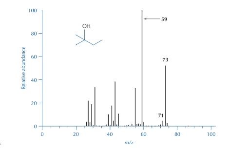
FIGURE 23.13 Mass spectrum of 2-methyl-2-butanol.
