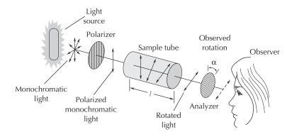
FIGURE 16.4 Schematic diagram of a polarimeter.
