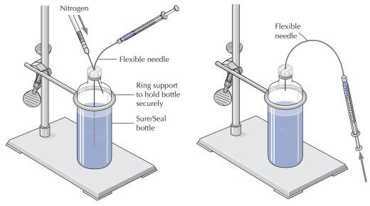
(a) Filling syringe using nitrogen pressure
