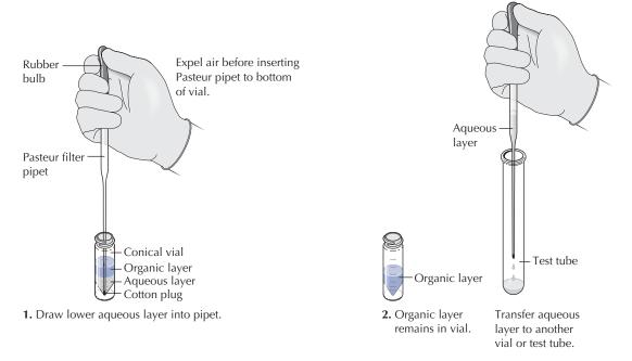
FIGURE 11.9 Washing an organic phase less dense than water.
