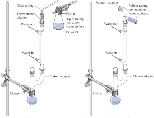
(a) Gas trap attached to reaction apparatus
