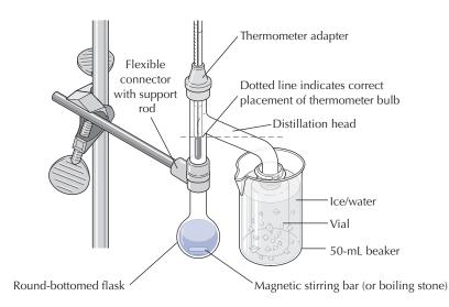
**FIGURE 13.13** Williamson microscale distillation apparatus. flask and clamp the rod to a vertical support rod or ring stand. Fit the flexible thermometer adapter to the top of the distilling head and carefully push a thermometer through the adapter.
