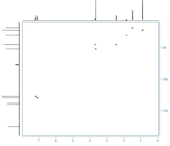
FIGURE 22.22 2D (C,H) COSY spectrum of the methyl ester of ibuprofen.
