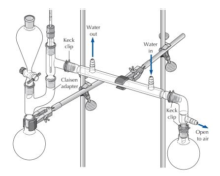
**FIGURE 13.21** Steam distillation apparatus.
