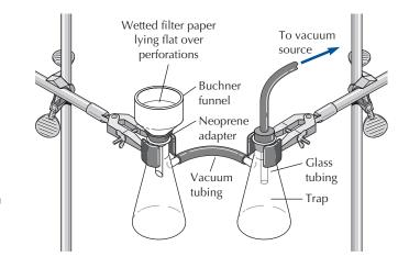
vacuum system or vacuum pump, the trap flask keeps any overflow from the filter flask out of the vacuum line.
