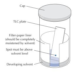
**FIGURE 17.5** Developing a TLC plate.
