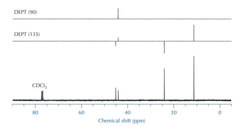
**FIGURE 25.13** 90-MHz <sup>13</sup>C NMR, DEPT(90), and DEPT(135) spectra of unknown compound for problem 7.
