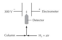
FIGURE 19.6 Flame ionization detector.
