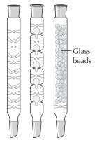
**FIGURE 13.14** Examples of fractionating columns.
