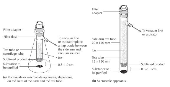
FIGURE 16.1 Two simple apparatuses for sublimation.
