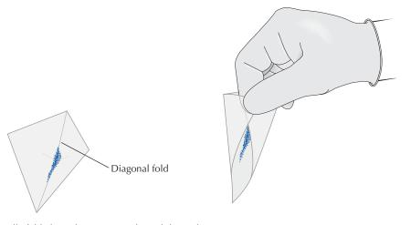
(a) Diagonally folded weighing paper with a solid sample
