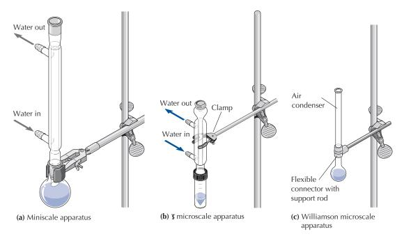
FIGURE 7.1 Apparatus for simple reflux.
