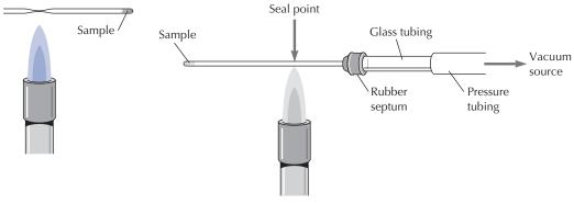
(a) Sealing a capillary tube
