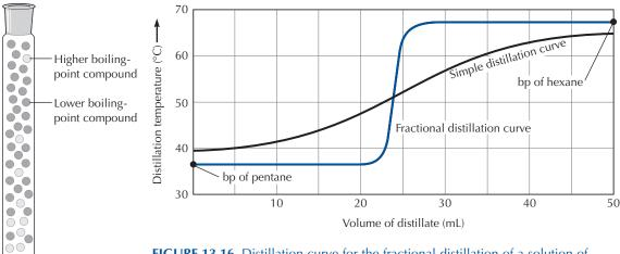
**FIGURE 13.16** Distillation curve for the fractional distillation of a solution of pentane and hexane. The dashed line represents the distillation curve for a simple distillation of the same solution.
