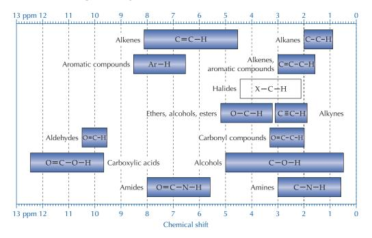
**FIGURE 21.12** Approximate regions of chemical shifts for different types of protons in organic compounds.
