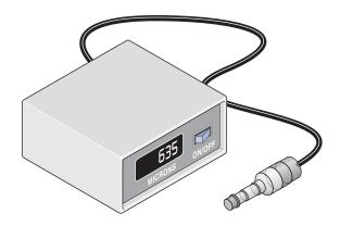
**FIGURE 13.25** Digital, nonmercury vacuum gauge.
