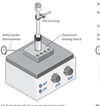
(a) Typical standard taper reaction apparatus with a conical vial and an air condenser
